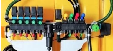
Fig. 41. Distributor equipped with additional solenoid valves for switching individual sprayer sections on/off with Control Panel 7®.
