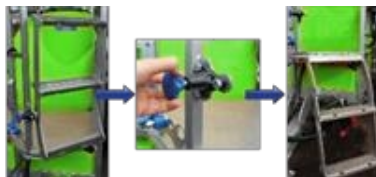
Fig. 29. Opening the ladder providing access to the platform
