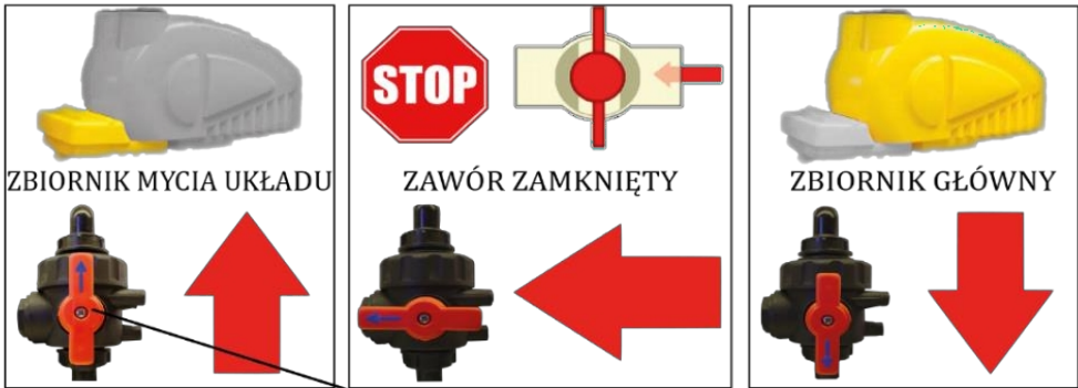
Fig. 35. Three-way valve operation. 1. Knob.
