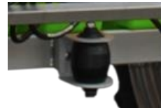
Fig. 24. Field boom vibration shock absorber
