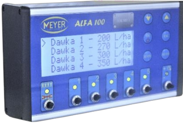
Fig. 45. Alfa 100 computer. Optional Control Panel 4 controller. Functions: On/Off, pressure adjustment, turn each section on/off separately, dose adjusted to tractor/sprayer speed, memory. It is clear, easy to use, and signals when driving too fast/slow, which prevents the correct dose from being applied.
