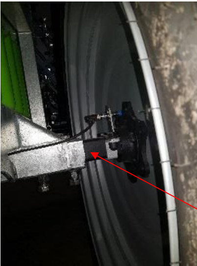
Fig. 36. Wheel calibration sensor
