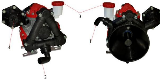
Fig. 44. Tolveri PU-3/140 pump. 1. Discharge connection. 2. Suction connection. 3. Oil filler with level indicator. 4. Air tank vent. Correct pressure: 1/3 of the pump's working pressure – no more than 105 bar.
