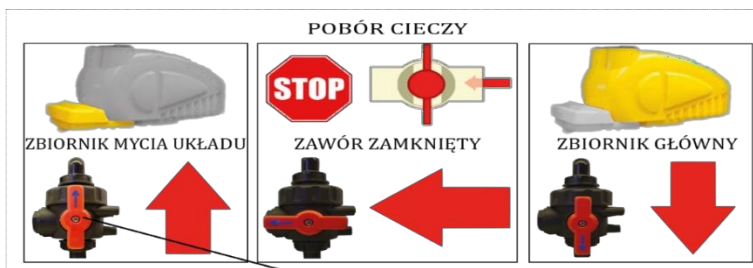
Fig. 30. Operation of the three-way valve. 1. Knob.
