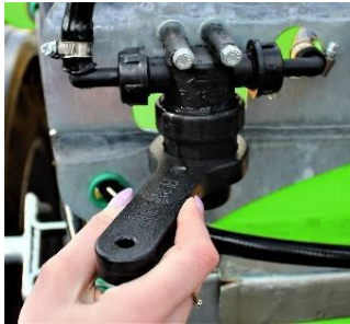
Fig. 49. In-line filter 1. In-line filter body. 2. 45° elbow. 3. In-line filter screen. 4. Filter housing
