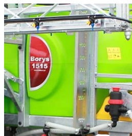
Fig. 40. Main tank water gauge
