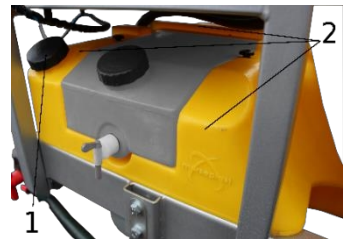
Fig. 9. 1. Water inlet for system flushing. 2. System wash water tank.
