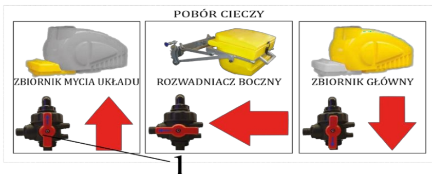
Fig. 31. Operation of the four-way valve. 1. Knob.
