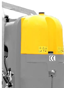
Fig. 4.2. System wash water tank
