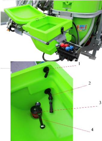
Fig. 8. Side diluter 1- liquid inlet, 2- hydraulic agitator, 3- drain with sieve, 4- rotary nozzle
