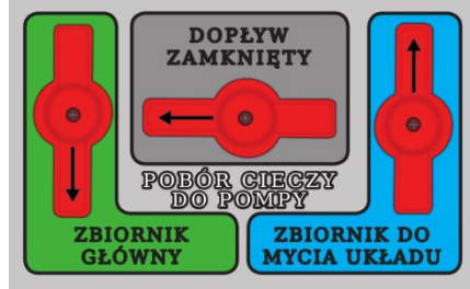
Fig. 21. Operation of the three-way valve.
